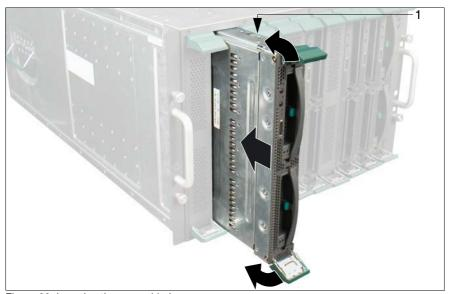
Figure 32: Inserting the server blade
